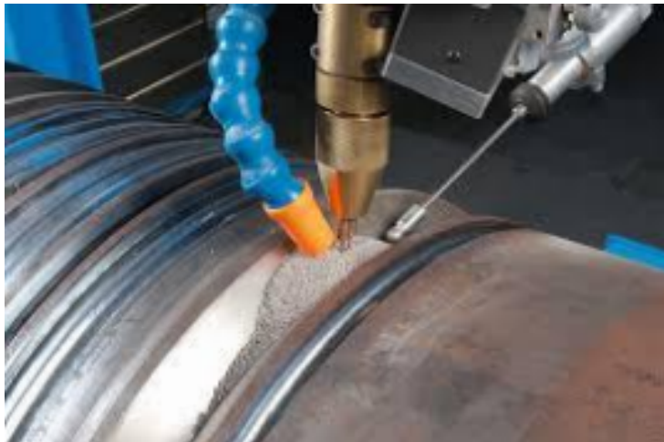
Figure 10 – Submerged Arc Welding (SAW) being used to join pipelines and industrial components.
