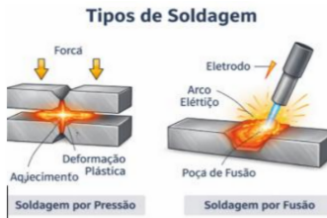
Figure 1 – Types of Welding
