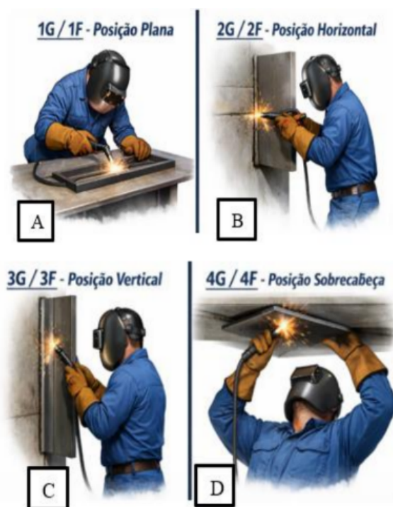
Figure 6 – Shielded Metal Arc Welding (SMAW) Welding Positions.
